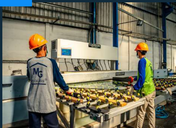
Horizontal Single Edger Line Ukuran maksimum 4200 x (any size) mm
