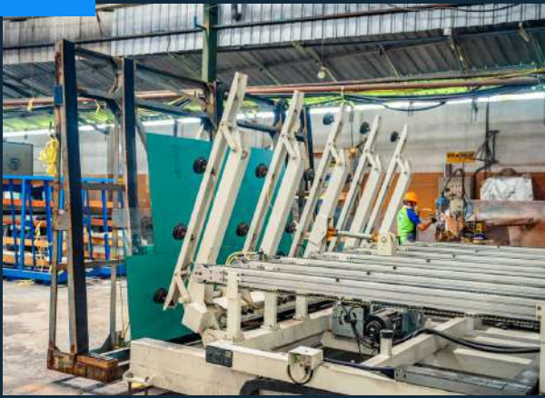
Fully Automatic Double Edger Line Ukuran maksimum 4500 x 2500 mm
